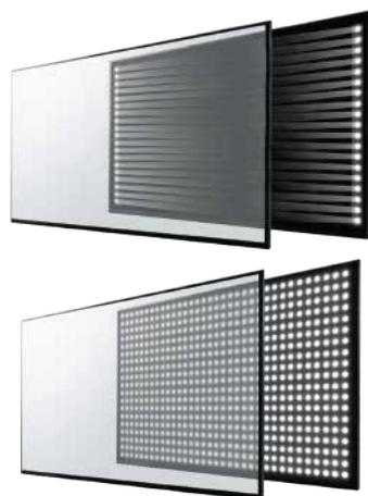
Top: Edge backlight method. Bottom: Full-array backlight method
